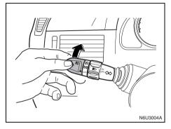
The exterior lamp band has three positions:
